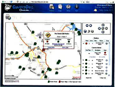
OmniSite's GuardDog web interface provides simple web navigation for monitoring pump stations.
